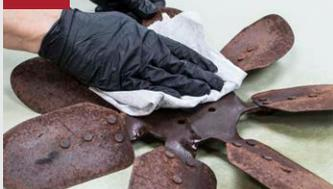
Remove loose scale with a wire brush. Clean with **SEM Solve** to remove oil, grease and dirt. Blow off with compressed air.
