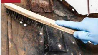
Remove loose scale with a wire brush. Clean with **SEM Solve** to remove oil, grease and dirt. Blow off with compressed air.
