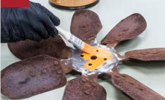
Apply 2 – 3 medium wet coats of **Rust Shield** with a brush or spray gun allowing a 3 – 5 minute flash time between coats. Maximum rust protection is achieved from thicker applications. Allow final coat to cure 24 – 48 hours before returning part to service.
