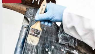
Apply 2 – 3 light coats of **Rust Seal** 5 – 10 minutes apart. Do not apply to sand blasted or painted areas. Allow to dry fully. **Rust Seal** does not require a top coat unless exposed to outdoor conditions. Body filler and top coat can be used after **Rust Seal** has fully dried.
