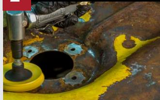
Remove loose rust scale by sanding, grinding or using a wire brush. Removing additional rust will result in a better final appearance. Abrade other surfaces with P180 grit. Blow off and re-clean with **SEM Solve**. Repeat until surface is free of contaminants.
