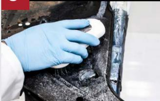
After conversion or removal, rinse treated areas using a brush with clean water to remove any **Rust Mort** that isn't dry. Dry thoroughly to avoid flash rusting. Proceed with body filler if needed, then topcoat.
