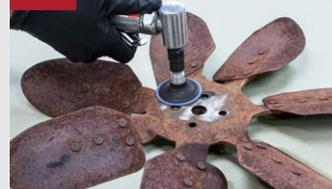
Remove loose paint and rust scale by sanding, grinding, or using a wire brush. Removing additional rust will result in a better final appearance. Sand painted areas with P220 grit. Blow off surface and clean again with **SEM Solve** or **XXX Universal Surface Cleaner**.
