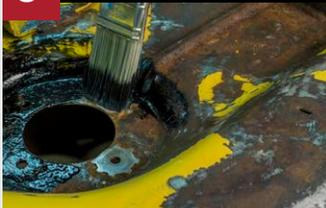
Apply 2 medium coats of **Rust Trap** with a brush or spray gun. First coat should not achieve full coverage and second coat should be applied in the same manner while first coat is still wet. Allow final coat to cure for 8 – 24 hours before returning part to service.
