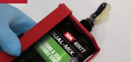
Place **Dual-Mix Sound & Seal Sprayable Coating** into **Universal Pneumatic Applicator**. Equalize cartridge until sides dispense equally. Attach **Quick Spray System** to cartridge.
