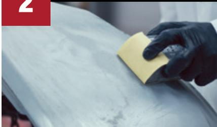
Apply **Guide Coat Black** or **Premium Powder Guide Coat** to dried primer. Sand with P320 – P400 grit. Finish sanding with P600 grit.
