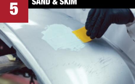
Sand with P80 grit. Finish with P180 grit. If needed, use a skim coat of **BUMPER BITE™ Flexible Glaze**, then sand with P180 – P320 grit.
