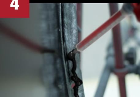
Apply 3/8" – 1/2" diameter bead of **Dual-Mix Multi-Purpose Panel Adhesive** or **Dual-Mix Weld-Bond Adhesive** to both surfaces. Use enough material to completely fill the joint when parts are clamped. Tool with a spreader or acid brush. Cover all exposed bare metal.
