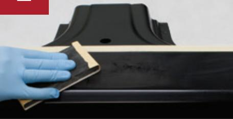
Sand primer with P180 grit. Sand bare metal with P80 grit. Blow off and tack clean. Re-clean with **SEM Solve** or **XXX Universal Surface Cleaner**. Wipe clean in one direction with clean, lint-free cloth.
