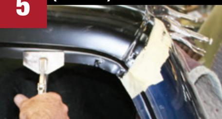
Clamp panel in place. Do not over clamp. Wipe away excess material.
