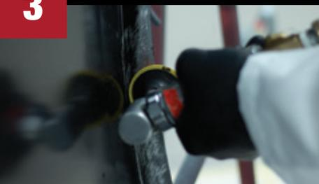
Clean with **SEM Solve** or **XXX Universal Surface Cleaner**. Grind mating flanges with a P36 grit grinding disc at low speed for aggressive grind mark. Remove any adhesive or protective coatings.
