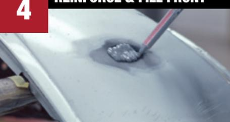
Remove tape from front. Fill front with **Dual-Mix Multi-Plastic Repair Material** or **Dual-Mix Problem Plastic Repair Material**. Spread material firmly and build up higher than panel to allow for sanding.
