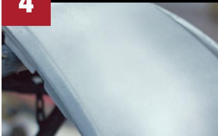
Apply **BUMPER COATER™** flexible coating or **FACTORY PACK™** basecoat as per instructions.
