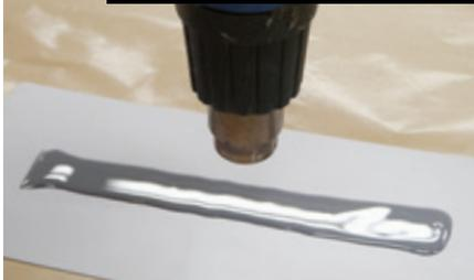
Apply **SEM 2K** seam sealer. Immediately smooth or tool seam sealer to match OEM texture.
