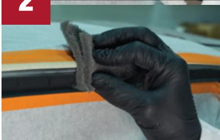
**BARE METAL SURFACES:** Sand with P80 grit. Blow off and tack clean to remove lint and dust. Re-clean with **SEM Solve** or **XXX Universal Surface Cleaner**.
