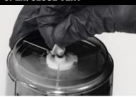
Open vent in liner for most spray applications.
