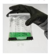
Competitor B's liner system created a major restriction in the liner, showing that it would starve the spray gun of fluid and create inconsistent flow. The final 8 oz. of fluid in the cup would not flow out of the cup.
