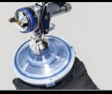
Press adapter onto assembled cup. Align locking tabs on adapter to corresponding tabs on lid.
