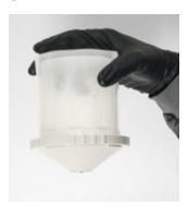
Competitor A's vented hard cup system dispensed all fluid in the cup but produced a major restriction and an inconsistent "glugging" paint flow.
