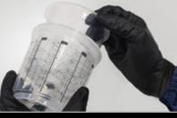
Insert liner into hard cup. Make sure to align vent tabs on liner with slots in bottom of hard cup.
